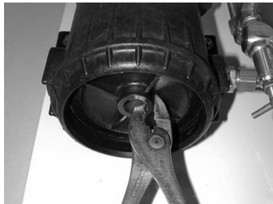
Figure 6: Pulling End Plug
