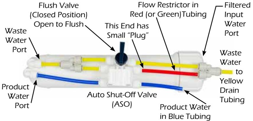
**NOTE: If Flush Valve is OPEN, product water cannot be produced.**
