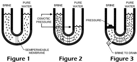
Household water pressure is used to force tap water through the semipermeable RO membrane. The membrane only allows the purest of water molecules to pass through it while over 98% of most salts and other impurities are rejected and automatically rinsed from the membrane down the drain.
