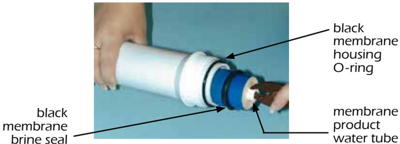
6. Remove the black housing O-ring (Fig. D). Wash the empty housing with soapy water. Rinse thoroughly with hot, clean water.
