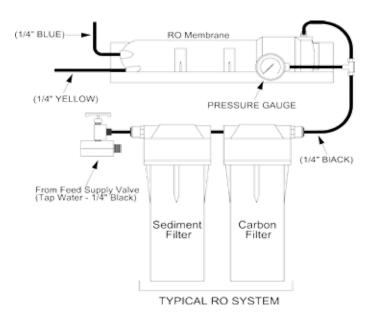
Figure 1: Installation of Pressure Gauge Kit.
